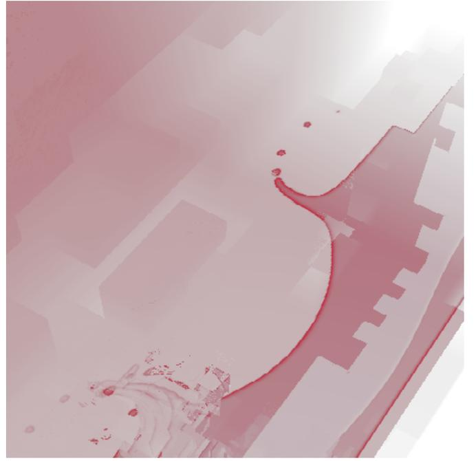
Fig. 5. A zoomed-in view of the STP dataset (about 25M tetrahedra) during interaction. Significant performance improvements are made by frustum-culling the geometry on the server. Here, 50% of the geometry is culled during the progression.
