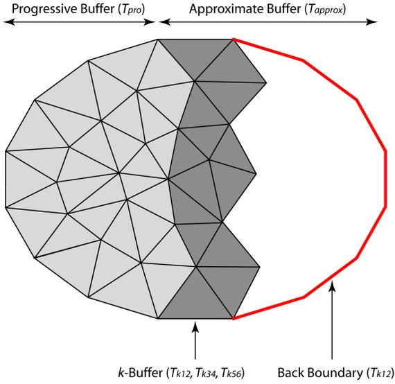
Fig. 3. The progressive volume renderer on the client. A progressive buffer is maintained between steps and an approximate buffer is created to fill the unknown region of the mesh.
