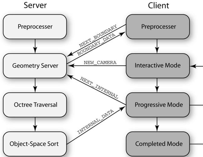
Fig. 2. The client-server architecture. Communication between the client and the server is shown with annotated arrows.
